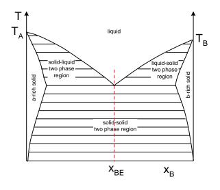
Figure 6: Eutectic Phase diagram
