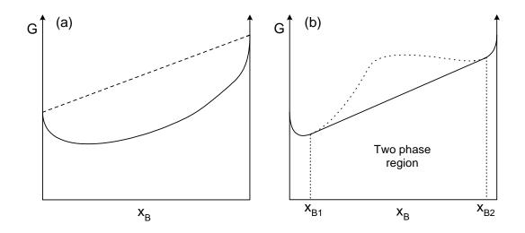
Figure 1: (a)  $G(x_B)$  for an ideal mixture ( $\varepsilon_{mix} = 0$ ) or one with  $\varepsilon_{mix} < 0$ . (b)  $G(x_B)$  for  $\varepsilon_{mix}$  sufficiently positive and *T* sufficiently low that the entropy of mixing does not completely dominate. The dashed line in (a) is *G* for the unmixed state. In (b) convexity arguments show that we must replace the dotted portion of the curve by the common tangent.
