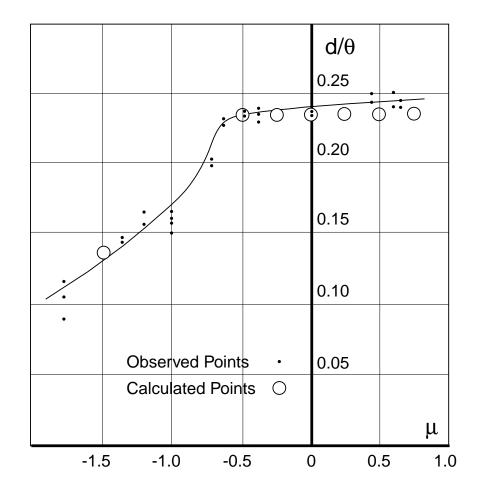
The outer and inner radii were  $r_0 = 4.04$  cm, and  $r_i = 3.80$  cm.  $\mu$  is the ratio of outer to inner rotation rates  $\Omega_2/\Omega_1$ . The vertical label  $d/\theta$  is the average width of a vortex in centimeters.
