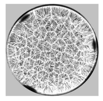
• The layer rapidly resolves itself into a number of *cells*, the motion being an ascension in the middle of the cell and a descension at the common boundary between a cell and its neighbours.
