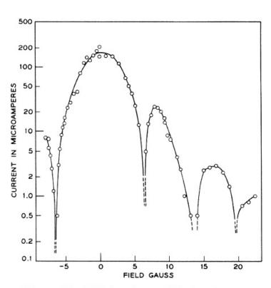
FIG. 3. The field dependence of the Josephson current in a Pb-I-Pb junction at 1.3  $^{\circ}K$ .
