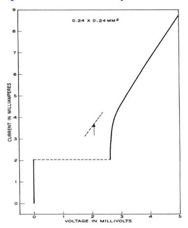
FIG. 1. Current-voltage characteristic for a Pb-I-Pb junction at 1.3°K. The arrow marks the predicted maximum magnitude of the Josephson current.
