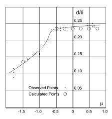
The outer and inner radii were  $r_0=4.04$  cm, and  $r_1=3.80$  cm.  $\mu$  is the ratio of outer to inner rotation rates  $\Omega_2/\Omega_1$ . The vertical label  $d/\theta$  is the average width of a vortex in centimeters.
