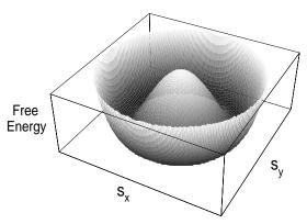
Rotation of s everywhere through any angle  $\Theta$  leads to an equivalent state (same free energy, etc.)
